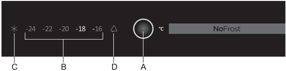
A Temperature adjustment and freezer boost key
