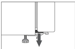
Spacers are fitted on the corners of the doors. Remove them and insert the supplied plugs into their slots (only in some models).
