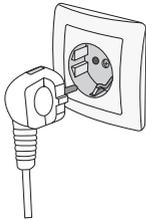
To **switch on** the appliance, plug the power cord into the power mains outlet.
