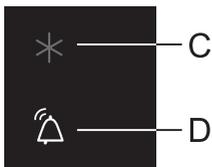
If the temperature inside the appliance is too high, acoustic alarm will be activated (intermittent tone) and the **D** symbol will flash.
